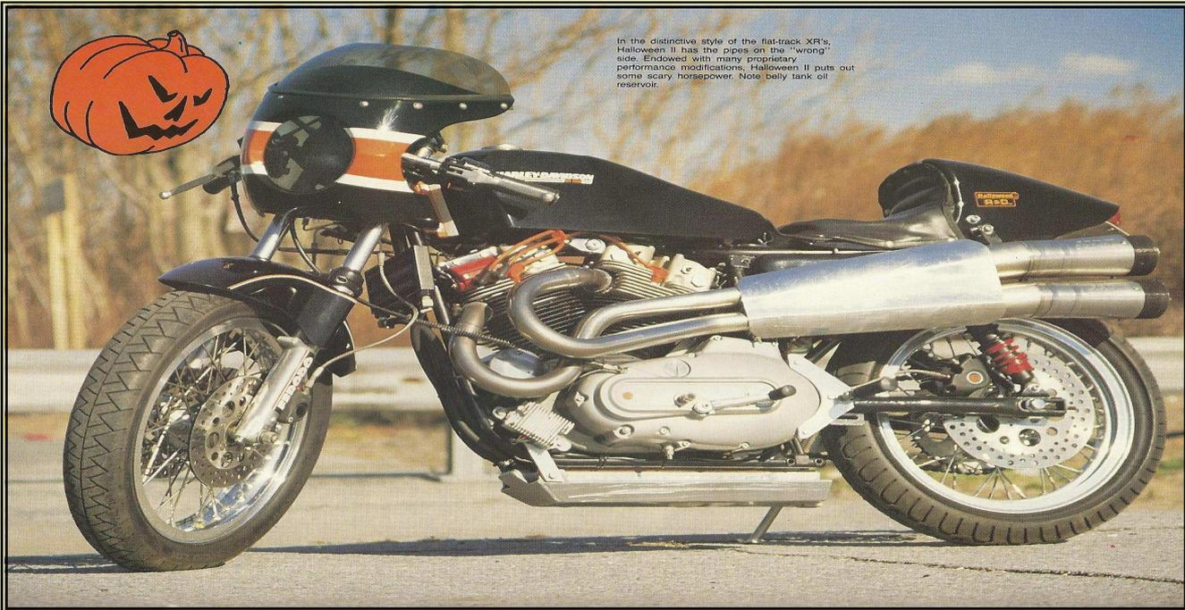
In the distinctive style of the flat-track XR's, Halloween II has the pipes on the "wrong" side. Endowed with many proprietary performance modifications, Halloween II puts out some scary horsepower. Note bally tank oil reservoir.
